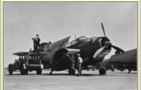
Life at NASFL: Mechanics loading TBF Wing guns. Photo taken in January, 1944.
