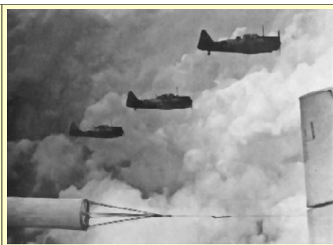
Sleeve target hooked to an Avenger. It trailed about 200 feet behind the airplane.
